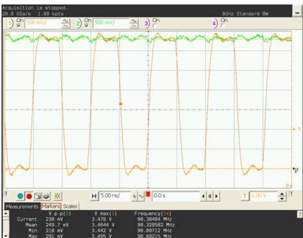
VDD=3.3V, Good decoupling:
