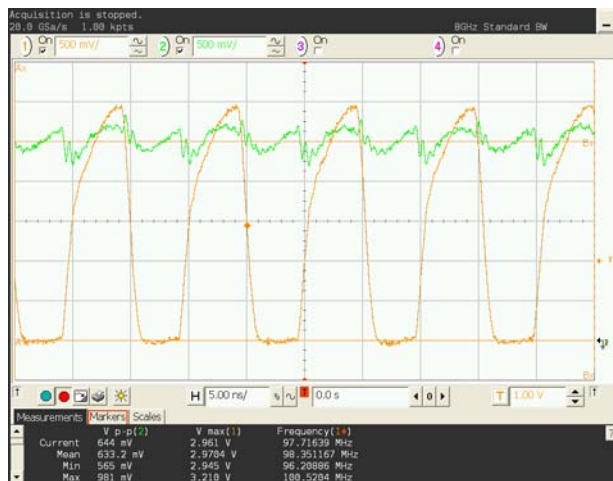
VDD=2.5V, Bad decoupling:
